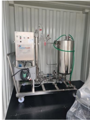
Figure 14: Austrian EcoSite nanofiltration membrane unit.
