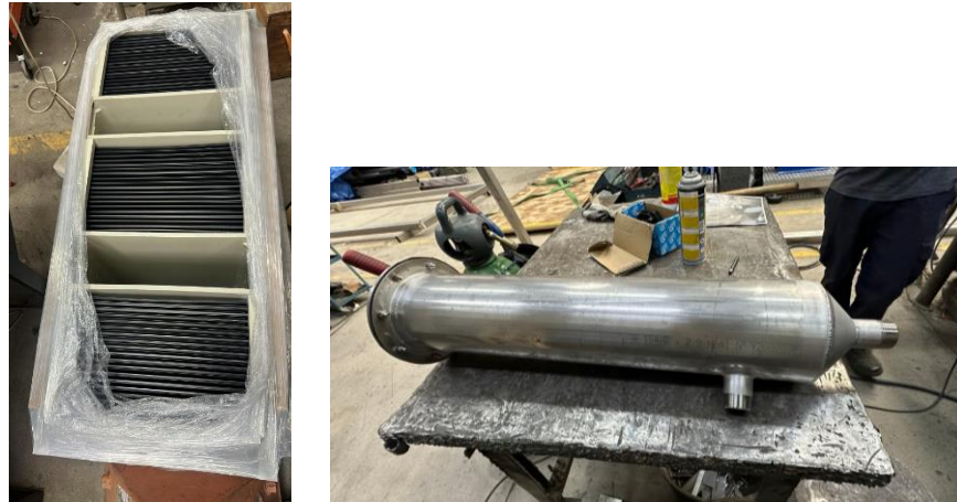
Figure 20: AlfaLaval membranes and degasser from the Danish EcoSite membrane unit.
