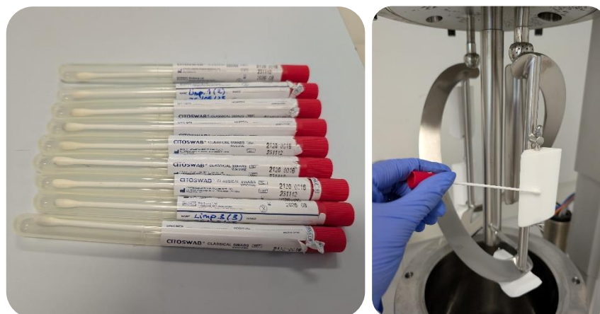
Figure 15. Measurement of reactor surfaces using swabs
