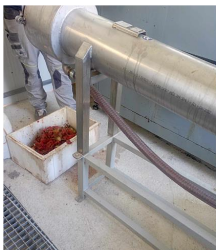
Figure 59. Extraction process taking place in the screw press of the Greek Ecosite
