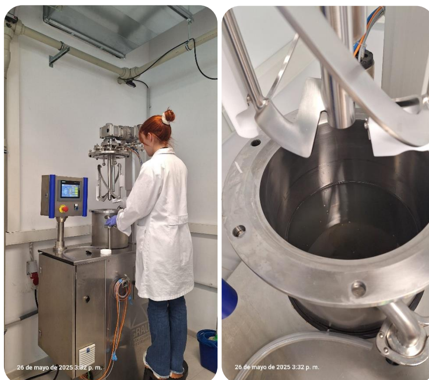
Figure 13. Photographs taken during the reactor cleaning validation test using treated wastewater.
