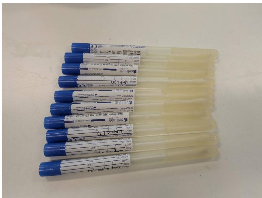
Figure 17. Photograph of the swabs employed during the reactor cleaning validation process using treated wastewater.
