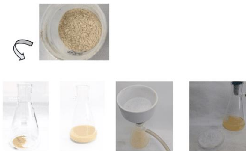
Figure 7. Experimental process followed for benzoic acid recrystallisation.
